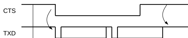
Figure 31-21. Transmitter Behavior when Operating with Hardware Handshaking
